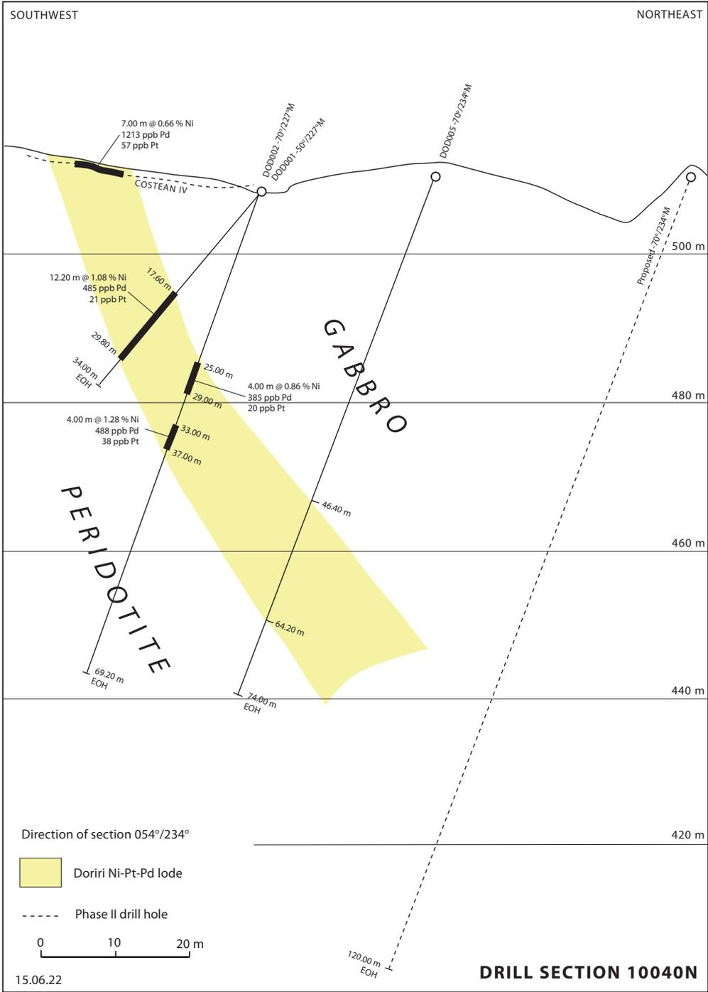
**Drill section 10040N showing existing holes DOD001 and DOD002, completed in 2012, present hole DOD005 and a proposed hole**
